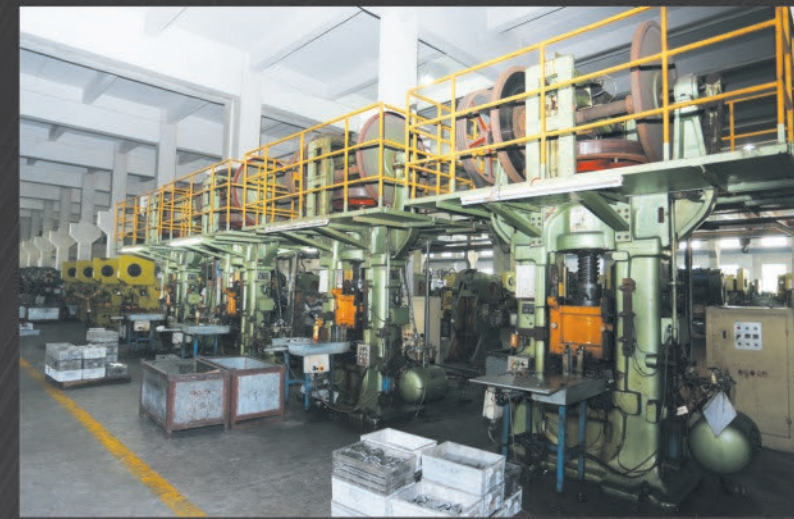
摩擦冲 20台 20 sets of friction screw press machine
