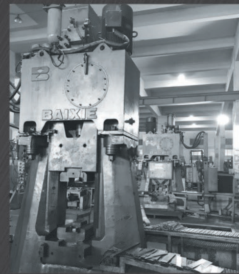
液压锻造 2组 2 sets of hydraulic forging hammer
