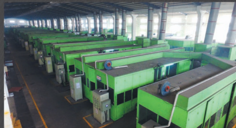
自动立式平抛 18组 18 sets of the automatic upright horizontal polishing machine
